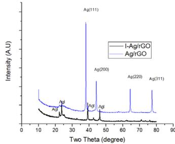
Fig 4. X-ray diffraction of Ag-GFs before and after iodine adsorption test
