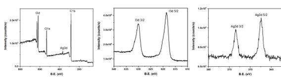
Fig 3. XPS of iodine adsorbed Ag-GFs
