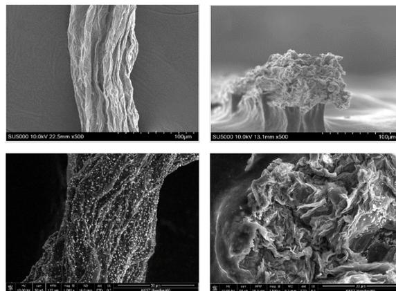
Fig. 1. Axis and cross-section SEM images of graphene fibers(up) and Ag-graphene fibers(down)
