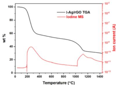
Fig 5. TGA-MS of iodine adsorbed Ag-GF
