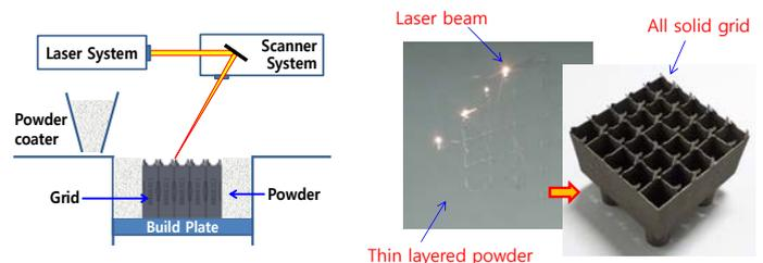
(a) PBF process concept (b) 3D printed grid
