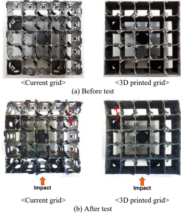
Fig. 6. Grid failure modes from dynamic crush test
