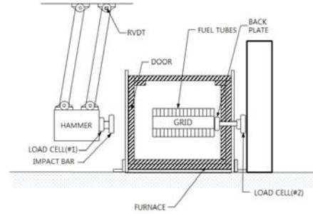
Fig. 5. Schematic of the dynamic crush test equipment
