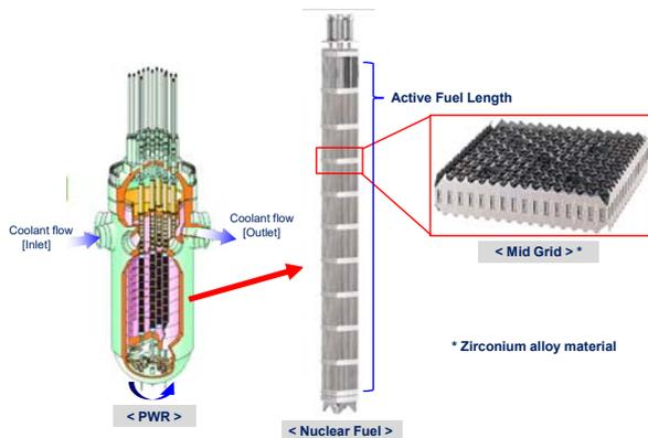
Fig. 1. Nuclear fuel and zirconium spacer grid
