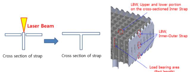
(a) LBW process concept (b) Conventional spacer grid
