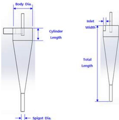
Fig. 1 Geometry of the hydrocyclone
