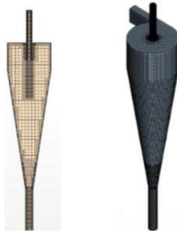
Fig. 2 Illustration of the CFD mesh
