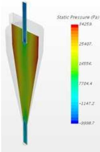
Fig. 3. Pressure distribution in a Cyclone
