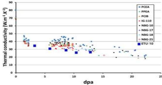
Figure 3. Irradiation-induced changes in TC of HFIR (ETU-10) and HFR (INNOGRAPH) [2][5].
