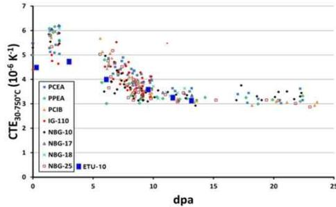
Figure 7. Comparison of CTE-dpa behaviors between the HFIR (ETU-10) and HTR (INNOGRAPH) [2][5]. Here, the HFIR (ETU-10) CTE-dpa data are overlapped on the HTR (INNOGRAPH) CTE-dpa data.
