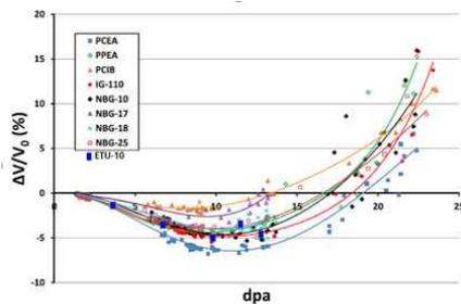
Figure 2. Comparison of the volume change behaviors with dose: Data from HFIR (ETU-10) were overlapped on the INNOGRAPH dimensional change data (HFR Innograph, Table 1) [2][5].
