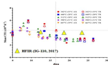
Figure 6. Comparison of CTE-dpa behaviors between HFIR (ETU-10) and HFIR (IG-110, 2017). Here, HFIR (IG-110, 2017) data are overlapped on HFIR (ETU-10) data for comparison [2][4].
