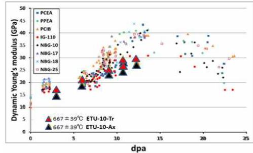
Figure 5. Comparison of DYM-dpa behaviors between HFIR (ETU-10) and HFR (INNOGRAPH). Here, HFIR (ETU-10) data are overlapped on HFR (INNOGRAPH) data for comparison [2][5].
