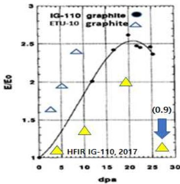
Figure 4. Comparison of irradiation-induced changes in DYM of HFIR (ETU-10), HFIR (IG-110, 2017), and HFIR (IG-110, 1996). Un-irradiated DYM of ETU-10 and IG-110 are 9.7-9.8 GPa and 9.1-10.2 GPa, respectively [2][3][4].
