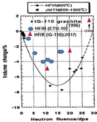
Figure 1. Comparison of volume change behaviors with neutron dose: HFIR (ETU-10), HFIR (IG-110, 1996), and HFIR (IG-110, 2017) [2][3][4].
