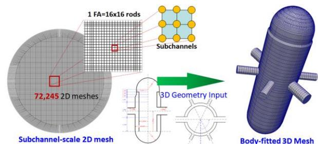
Fig. 1. Mesh generation of RPV using RVMesh-3D
