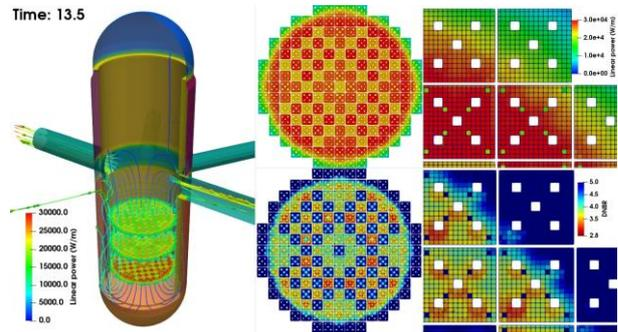
Fig. 3. Power and DNBR distribution prior to reactor trip
