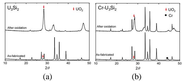
Fig. 5. XRD patterns of samples before and after the oxidation test. (a) Uncoated  $U_3Si_2$  (b) Cr-coated  $U_3Si_2$
