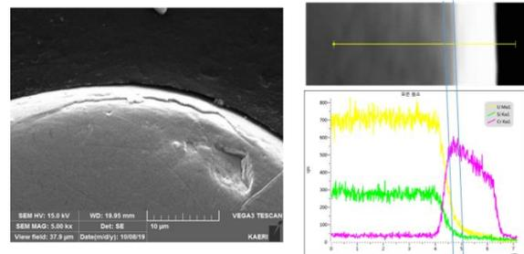
Fig. 2. (a) Cross-sectional image of Cr coated  $U_3Si_2$  (b) EDS line-scan profile across the coating layer
