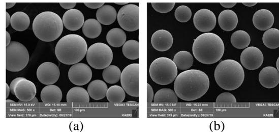
Fig. 1.  $U_3Si_2$  atomized particles. (a) As-fabricated particles (b) Cr-coated particles
