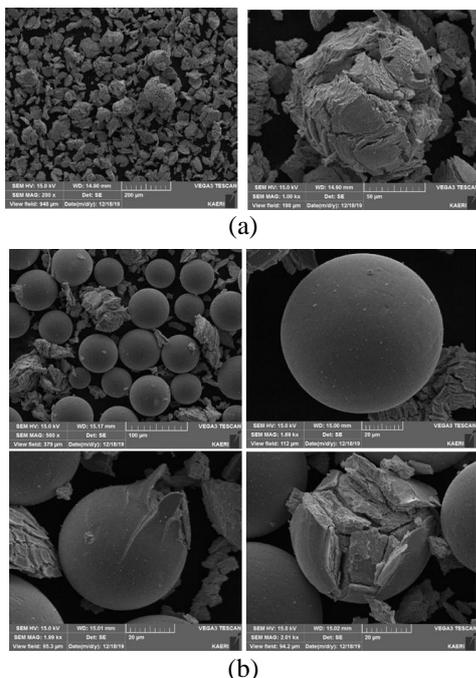
Fig. 3. Particle shape change after the oxidation test
