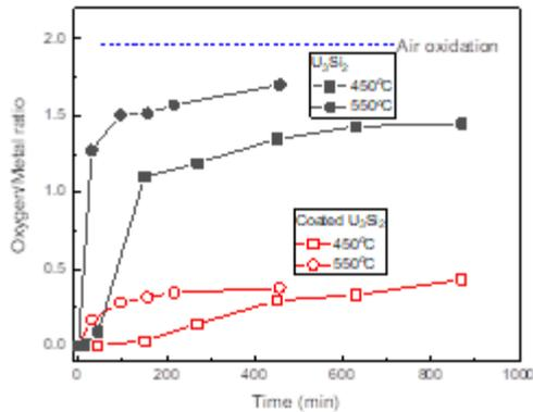
Fig. 3. Comparison of weight gain between sample particles during the annealing in the steam. The weight gain was converted to oxygen to metal ratio.
