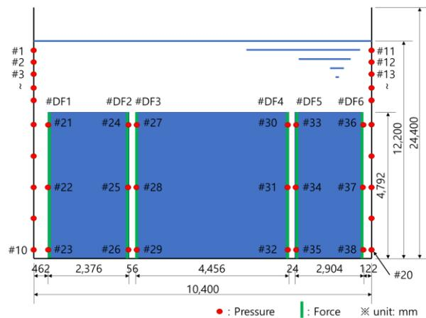
Fig. 1 Two-dimensional pool and rack for investigating the convective and impulsive effect of the coolant during seismic safety analysis
