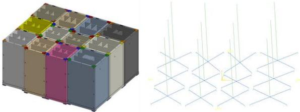
Fig. 3 Finite element models to analyze mechanical behaviors of racks using solid and beam elements
