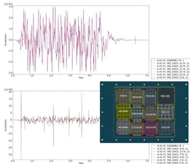
Fig. 5 Changes in acceleration during vibration of a spent fuel pool
