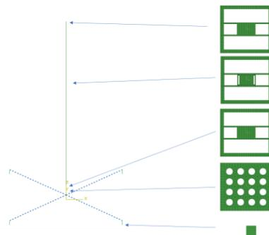
Fig. 2 Development of a finite element model of a simple rack using beam and warping elements
