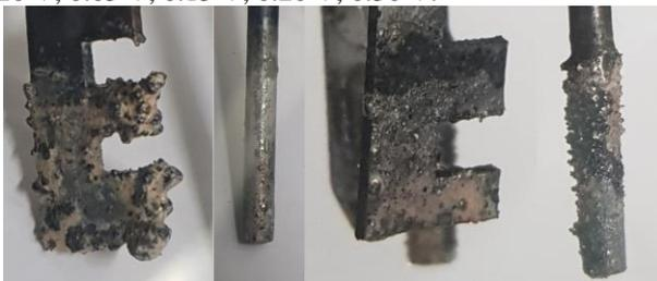
**Figure 2.** Ejected anode(left) and cathode(right) after experiment. Applied potential: 0.20 V, exchanged charge: 700 C, temperature: 500 °C
