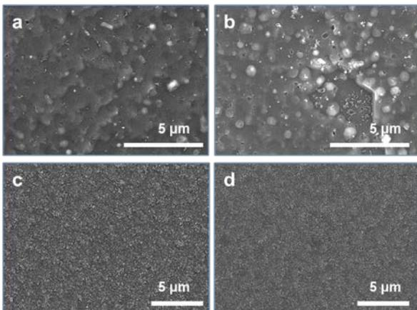
Fig. 2. SEM image of (a) GQDs on SiC and F-GQDs on SiC etched by fluorine plasma for (b)1 min, (c) 5min and (d) 10 min. (Magnification is 10k)
