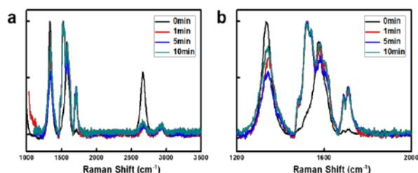
Fig. 4. Raman spectra of GQDs and F-GQDs etched by fluorine plasma for 1 min, 5min and 10 min. (a) Range from 1000-3500  $\text{cm}^{-1}$  and (b) 1200-2000  $\text{cm}^{-1}$
