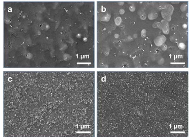
Fig. 3. SEM image of (a) GQDs on SiC and F-GQDs on SiC etched by fluorine plasma for (b) 1 min, (c) 5min and (d) 10 min at higher magnification. (Magnification is 20k)
