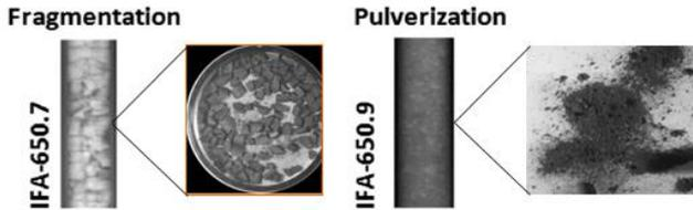
Fig. 1. Fuel fragmentation and pulverization in in-pile experiments
