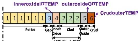
Fig. 4. Modification of thermal node for consideration of additional thermal barriers
