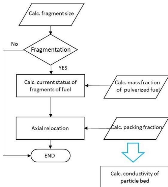
Fig. 2. Calculation flow of QT model
