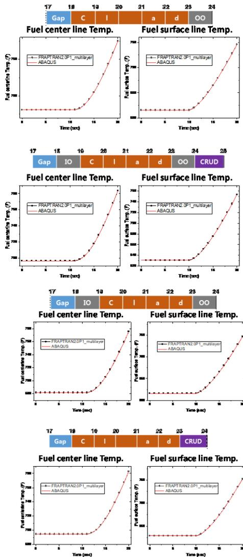
Fig. 6. Verification of thermal barrier model of MARS-KS/FRAPTRAN
