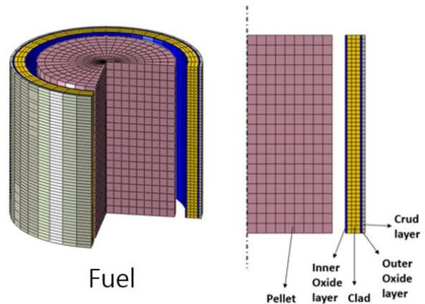
Fig. 3. Concept of oxide/CRUD thermal barrier of high burnup fuel
