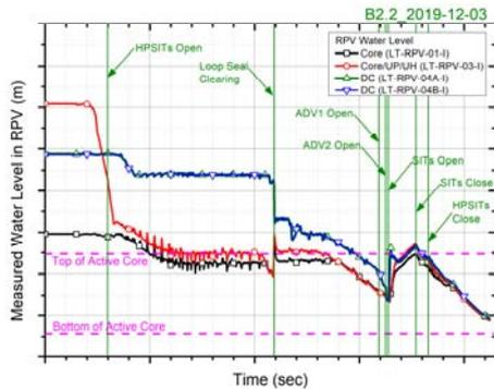
Fig. 8 Variation of measured water levels in the RPV vs. timing of major sequence of events
