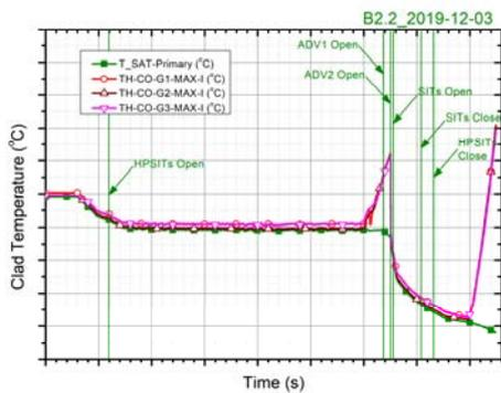
Fig. 9 Trends of the maximum clad temperatures
