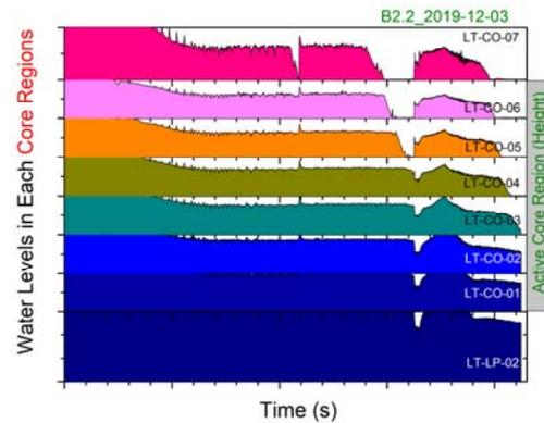
Fig. 6 Segmented water levels in the core region
