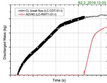
Fig. 1 Accumulated water mass from the CL break and the ADV2
