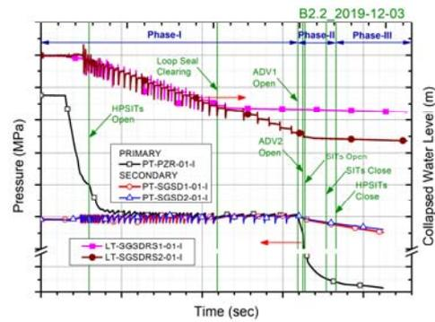
Fig. 5 System pressure trends with water levels in 2<sup>nd</sup>-side of SGs
