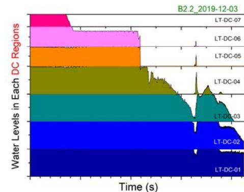
Fig. 7 Segmented water levels in the downcomer region
