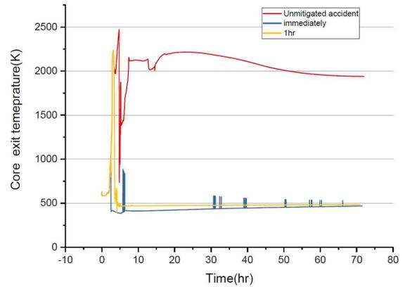
Fig. 4. Core exit temperature
