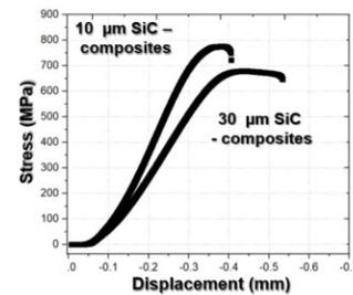
Fig. 2. Strain-stress curves of tested composites.
