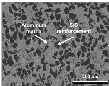
Fig. 1. The microstructure of fabricated composites.
