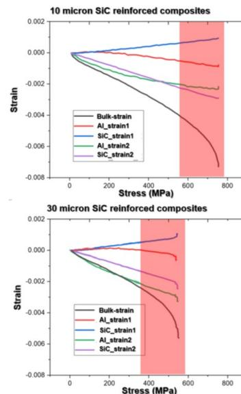
Fig. 3. Strain-stress curves measured by neutron diffraction.
