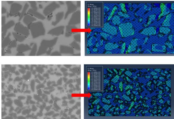
Fig. 4. Original microstructure images and the generated meshes with stress contour.
