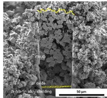
Fig. 3. SEM cross-section image of the sample in experiment U2 showing about 86.37  $\mu\text{m}$  thick, highly porous crud. Particle size decreases with increasing distance from the heated surface.
