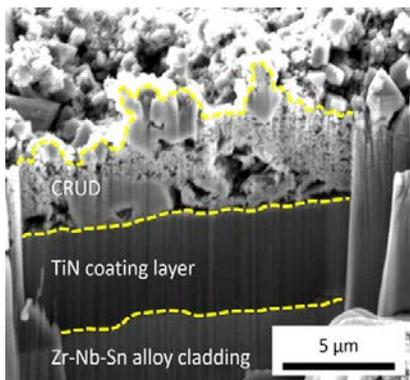
Fig. 5. SEM cross-section image of the sample in experiment T2 showing a thinner crud deposition layer than U2.
