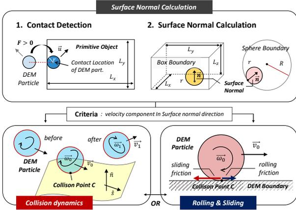
Fig. 4. New DEM wall boundary treatment model
