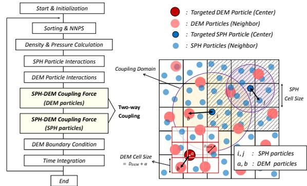
Fig. 6. Simplified algorithm of SPH-DEM phase coupling
