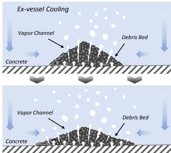
Fig. 1. Debris bed leveling behavior
