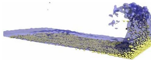
Fig. 8. 3D dam-break simulation of SPH-DEM coupled model
