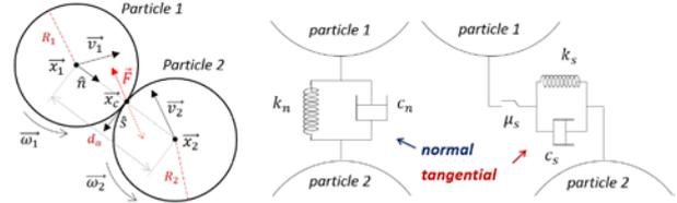
Fig. 3. Soft-sphere spring-dashpot collision model
