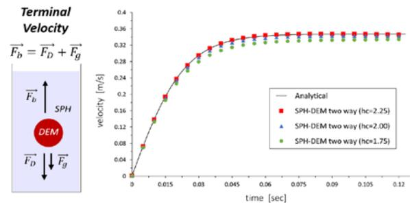
Fig. 7. Terminal velocity behavior of single DEM particle
