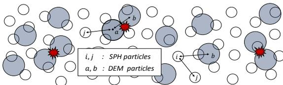
Fig. 5. Concept of SPH-DEM unresolved coupling
