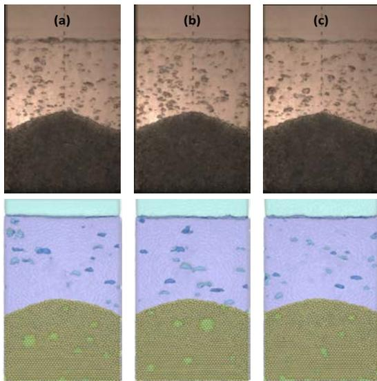
Fig. 9. Results of vapor-driven self-leveling simulation
