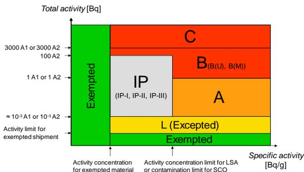
Fig. 3 Schematic description: Classification for transportation cask according to the activity and specific activity
