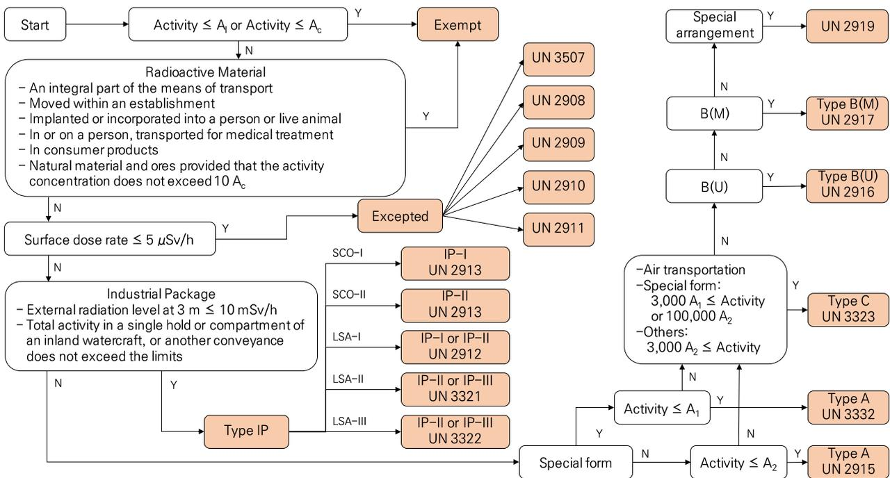
Fig. 5 Overall procedure to determine the types of transportation cask
