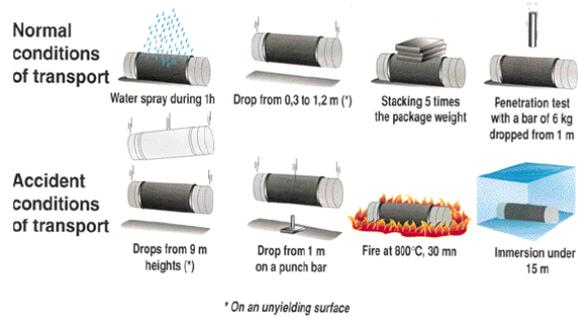
Fig. 4 Tests for the transportation cask
