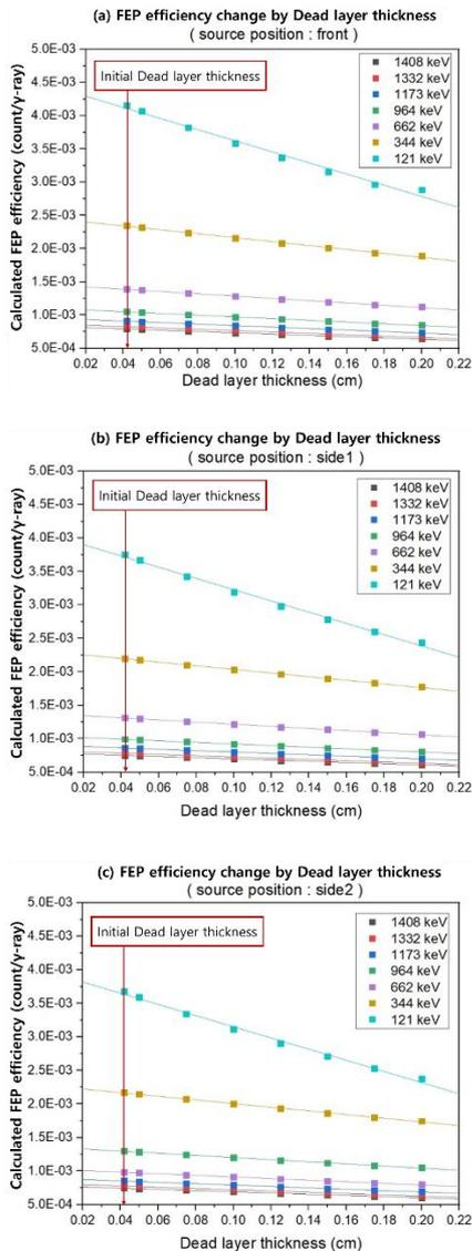
Figure 3 Approximation formula between the calculated FEP efficiency and the dead layer thickness (121~1408keV) (a) front (b) side1 (c) side2
