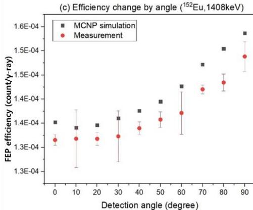
Figure 5 Comparison of calculated FEP efficiency (MCNP) and measured FEP efficiency by angle (a) <sup>137</sup>Cs (b) <sup>60</sup>Co (c) <sup>152</sup>Eu
