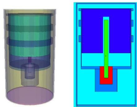
Figure 2 HPGe detector geometry in MCNP
