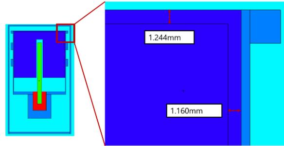
Figure 4 Adjusted geometry of HPGe detector
