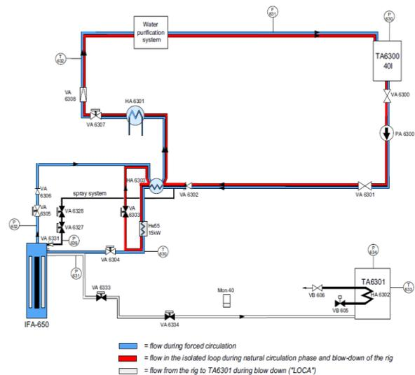
Fig. 1. System scheme of IFA-650.9 experiment [4]
