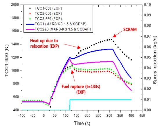
Fig. 3. Calculated fuel behavior of MARS-KS1.5&SCDAP against IFA-650.9 experimental results
