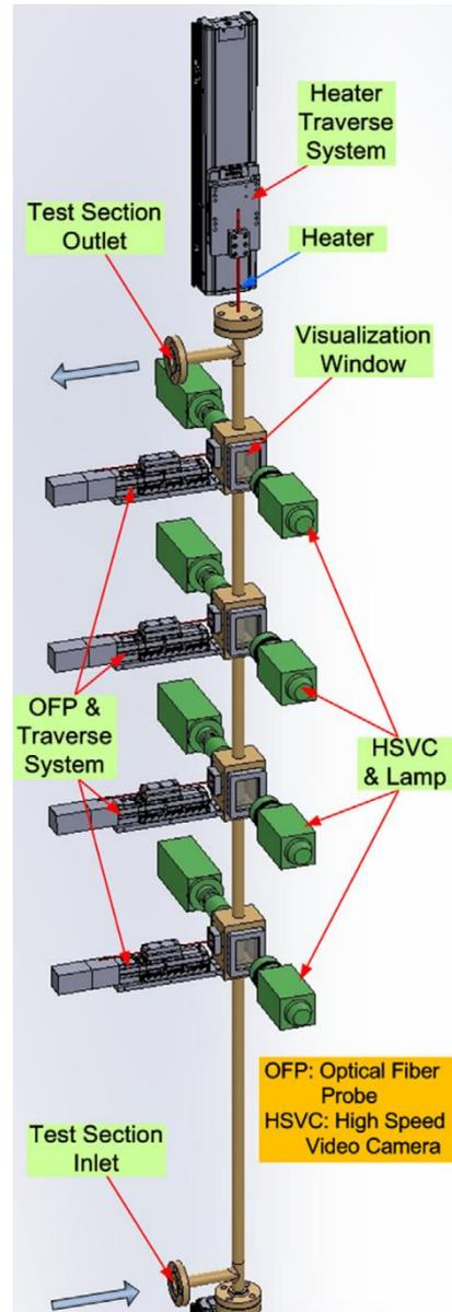
Fig. 1 Schematic of test channel
