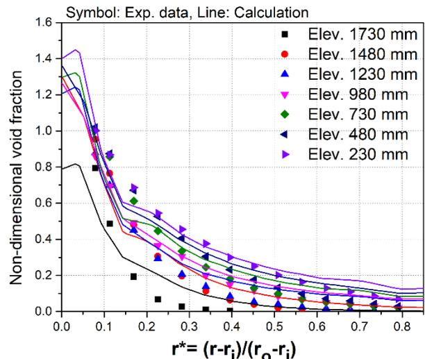
Fig. 3 Radial distribution of void fraction (Test-01)
