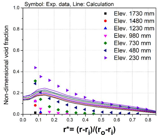
Fig. 6 Radial distribution of void fraction (Test-02)
