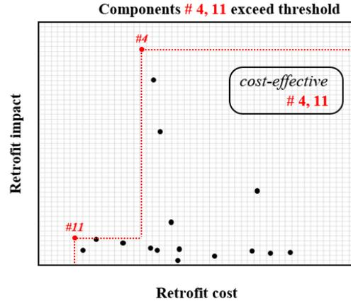
Fig. 4. Conceptual demonstration of selecting ‘cost-effective’ components
