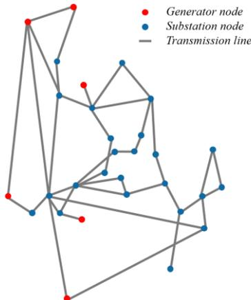
Fig. 6. Topological distributions of 30-bus system
