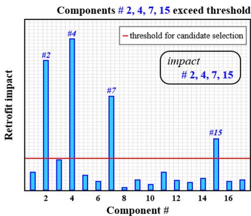
Fig. 3. Conceptual demonstration of selecting ‘impact’ components with high retrofit impact
