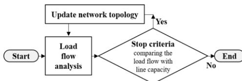
Fig. 1. The overload cascading model (Pahwa *et al.*, 2013)
