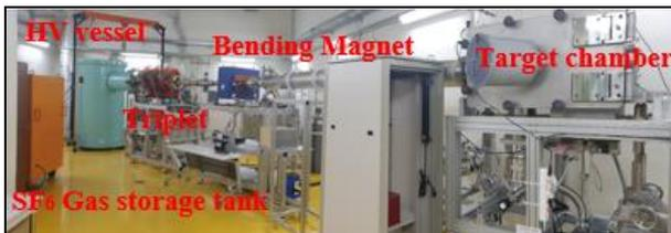
Figure.1. Layout of the accelerator
