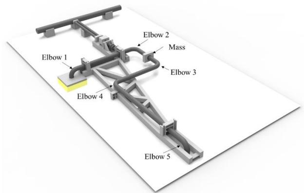
Fig. 2. Illustration of the piping system test facility [6]
