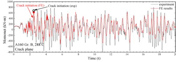
Fig. 4. Comparison of experimental moment data at crack plane pipe with simulated results.
