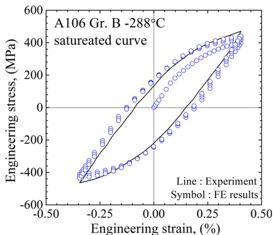
Fig.1. Comparison of experimental saturated stress-strain curve with simulated results under cyclic loading condition.
