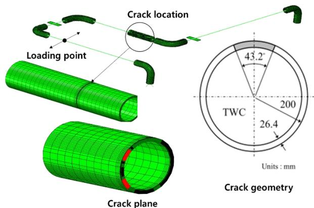
Fig. 3. Crack geometry of the through-wall cracked pipe..
