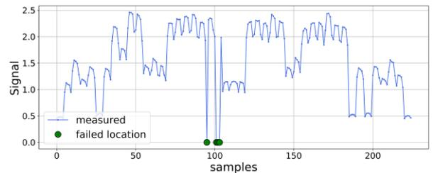
Fig. 4. ICI measurement with failed detectors
