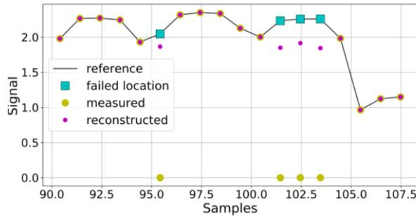
Fig. 7. Result of conventional  $\ell_1$ -reconstruction
