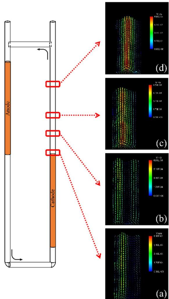
Fig. 4. Velocity profile at each observation points.
