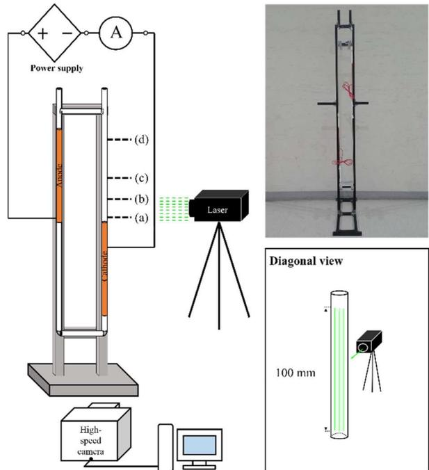
Fig. 1. Test apparatus and PIV setup.
