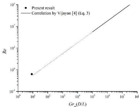
Fig. 3. Comparison of the present result with existing correlation.
