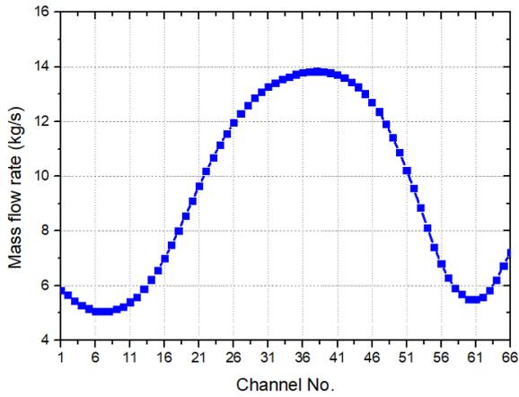
Fig. 3. Mass flow rate for each channel when no plate is added.
