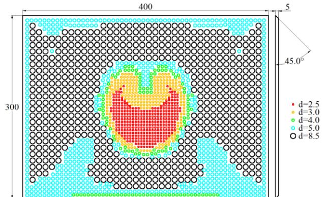
Fig. 6. The design of the perforated plate.
