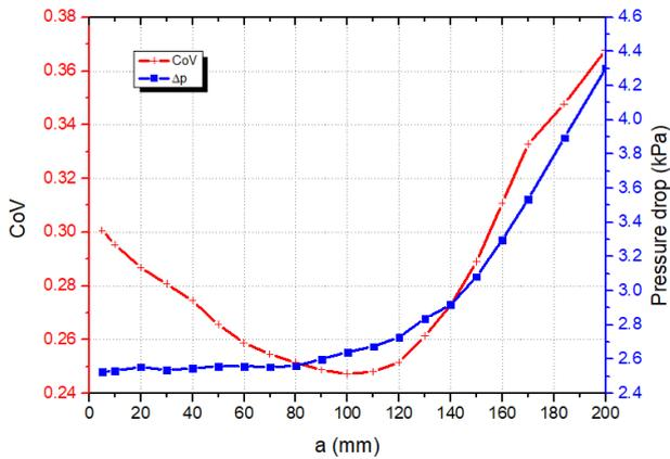
Fig. 4. The change of CoV and pressure according to distance a.
