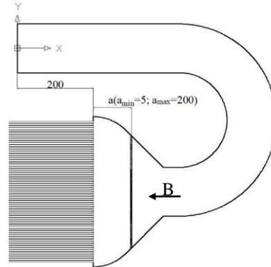
Fig.2. The perforated plate installed in the sodium channel inlet header
