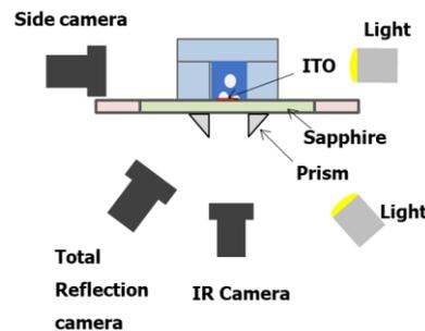
Fig. 2. Arrangement of cameras around the test section (top view)
