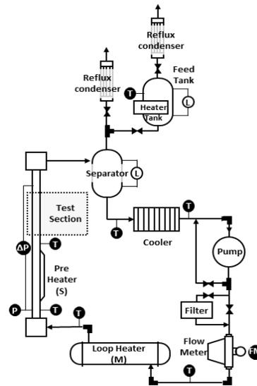
Fig. 1. Schematic for the DNB test loop
