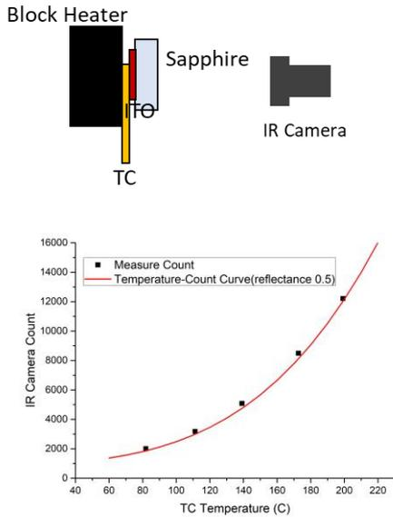
Fig. 3. Setup (top) and results (bottom) for calculation of sapphire-ITO reflectivity
