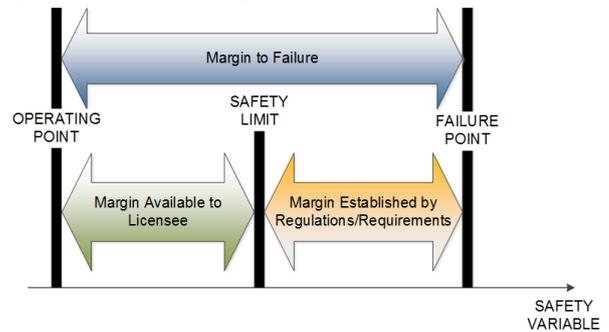
Fig. 2. SM and the safety limit (EPRI [1]).
