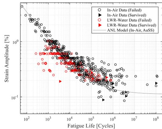
Figure 1 All fatigue data of Ni-base Alloys and welding materials extracted from NUREG/CR-6909, classified according to in-air/LWR-water environment and exact/right-censoring data.
