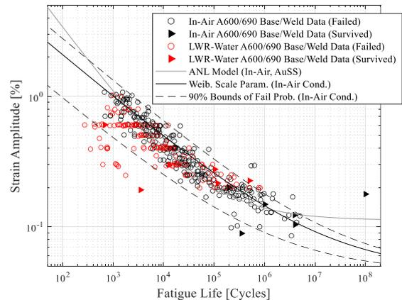
Figure 2 Result of Weibull-based probabilistic environmental fatigue life model.
