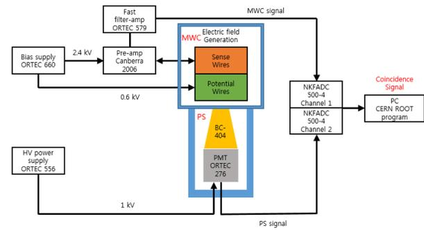
Fig. 2. The schematic diagram of the beta-spectrometer measurement system.
