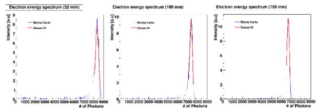
Fig. 6. The electron energy spectra according to the plastic scintillator thickness (blue line) and Gaussian fitting of the peaks (red line). The x-axis is the number of photons generated in the plastic scintillator corresponding to the energy. The y-axis is the intensity when the total area of the spectrum is 100.
