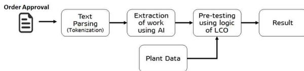
Fig. 3. The process of pre-testing for the work result
