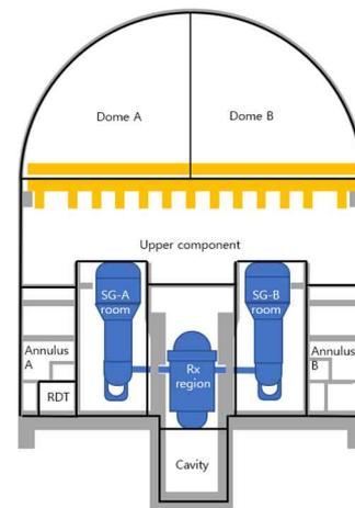
Fig. 1. The containment building nodes
