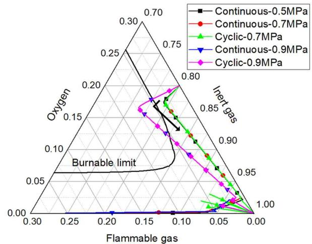
Fig. 3. The gas composition change in the CFVS vessel under LBLOCA.
