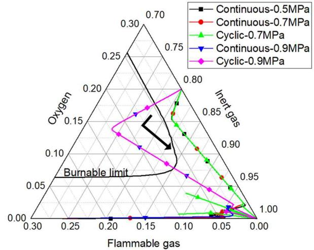
Fig. 2. The Gas composition change in the CFVS vessel under SBO.
