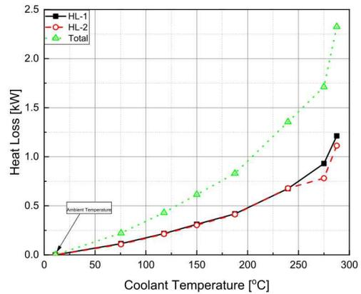
Fig. 6. Heat loss in hot legs
