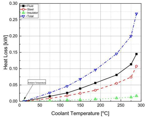
Fig. 5. Heat loss in zone 'C'
