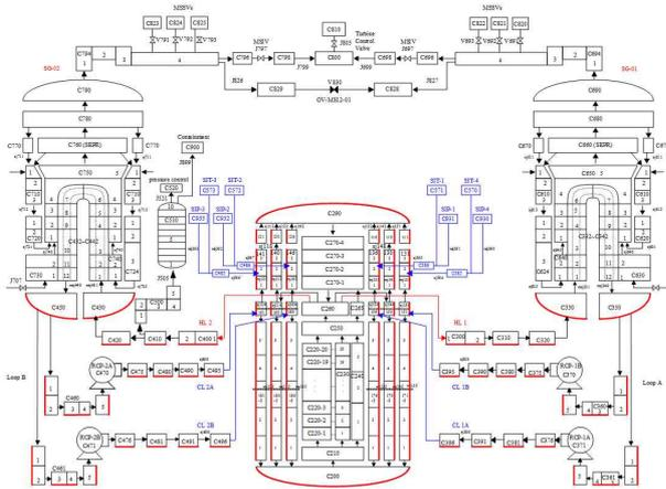
Fig. 8. Schematic diagram of ATLAS Facility
