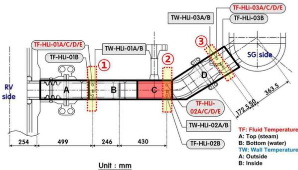
Fig. 3. Sectionalization of RCS piping
