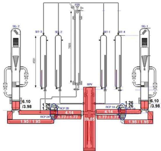
Fig. 7. Heat loss distribution in RCS
