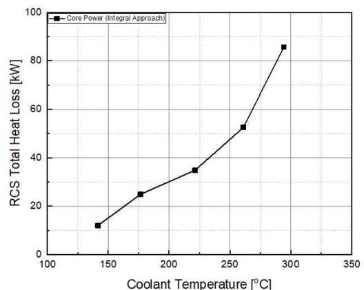
Fig. 2. Total heat loss in RCS
