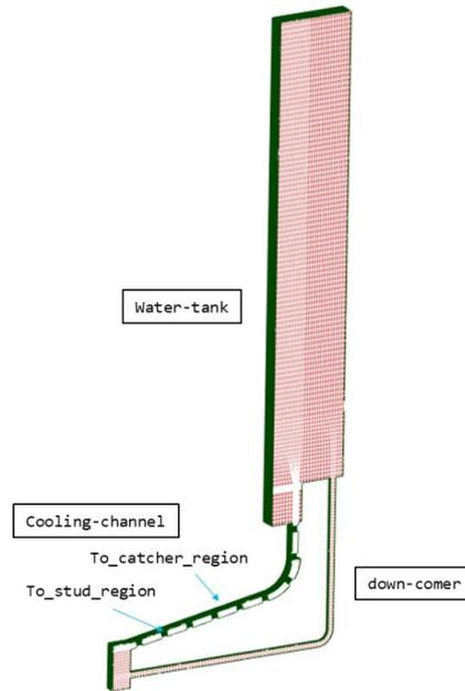
Fig. 4. Mesh system of CE-PECS test facility used for a preliminary analysis.
