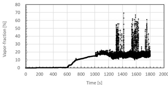
Fig. 5. Temporal volume-fraction of vapor going out cooling-channel of CE-PECS
