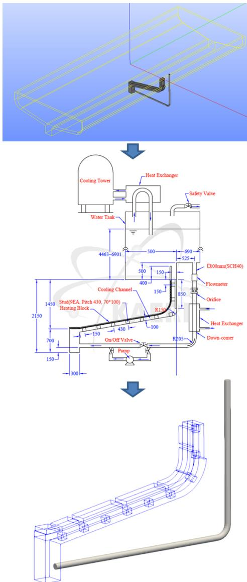
Fig. 3. CE-PECS test facility and geometrical modeling for a validation of the analytical method
