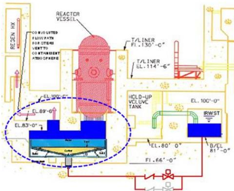
Fig. 1. Schematics of Core-Catcher for EU-APR1400 [2].
