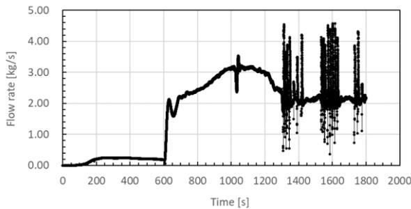
Fig. 4. Temporal flow rate of water flowing through down-comer of CE-PECS.
