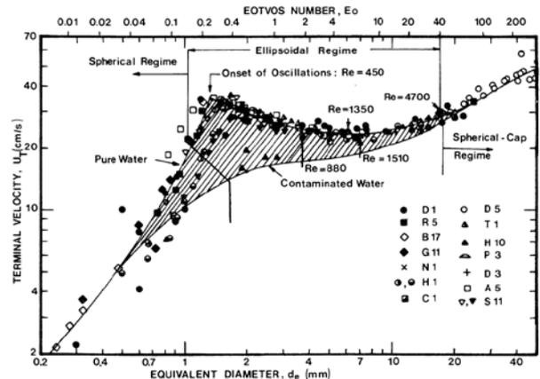
Fig. 4. Terminal velocity of clean water and contaminated water [6].
