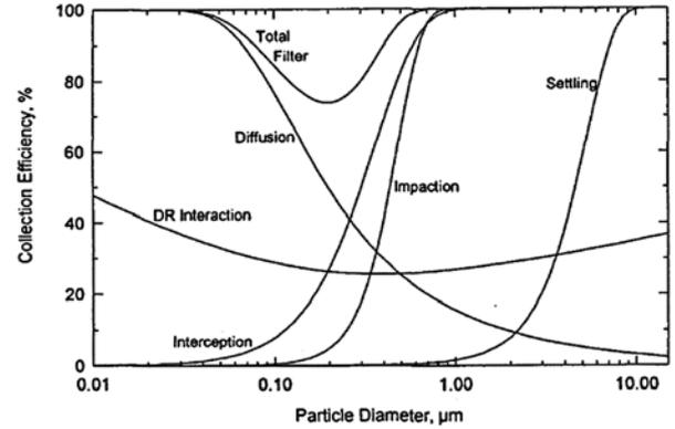
Fig. 1. Aerosol removal efficiency respect to particle size [4].
