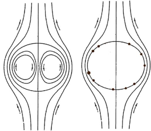
Fig. 2. Internal circulation in rising bubbles with or without contaminants [3].
