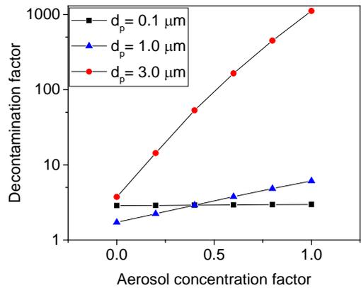
Fig. 3. DF calculation results for different ACF
