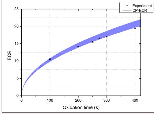
Fig. 2. Experimentally obtained ECR and CP correlation prediction at 1204 °C
