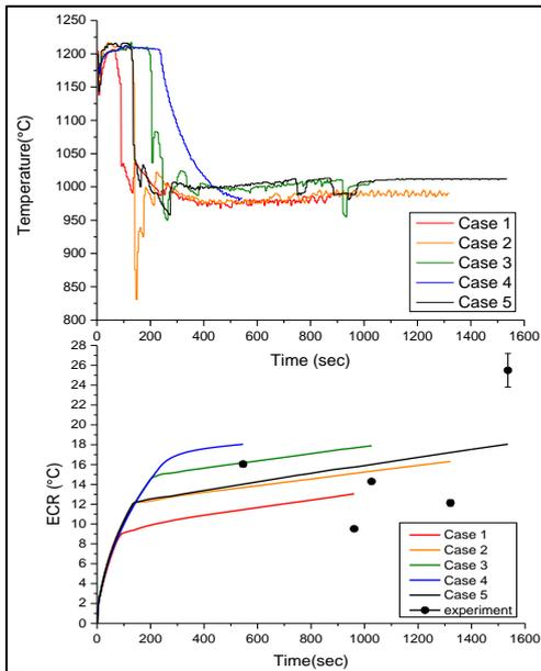
Fig.3. (a) tested temperature transience (b) calculated ECR with Cp correlation
