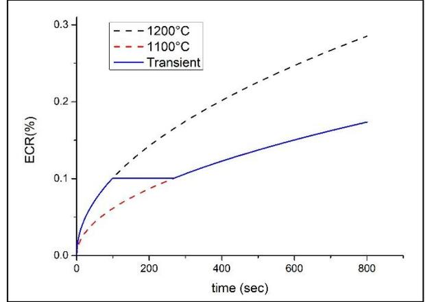
Fig.4. Schematic illustration of isothermal ECR used for non-isothermal transient calculation
