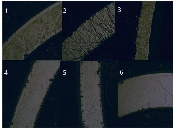
Fig.7. Optical Microscopy of non-isothermal specimens(No.9,12, and 14) and ECR corresponding isothermal specimens.
