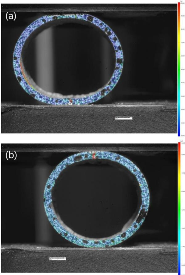
Fig.8. The first crack position(red color) difference of non-isothermal specimen(a) and corresponding isothermal specimen(b).
