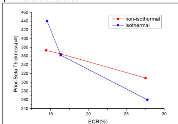
Fig.6. Prior-beta layer thicknesses of non-isothermal specimens(No.9,12, and 14) and ECR corresponding isothermal specimens.
