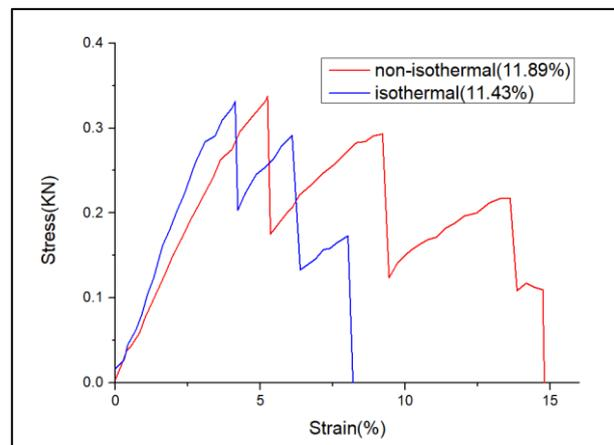
Fig.8. Strain-Stress curve of non-isothermal specimen of ECR 11.89%(specimen 6) and isothermal specimen of ECR 11.43%
