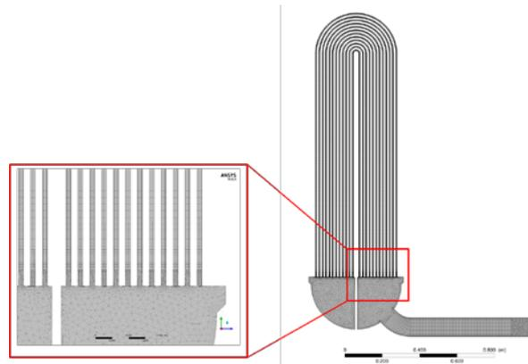
Fig. 3. Computational mesh without tube simplification
