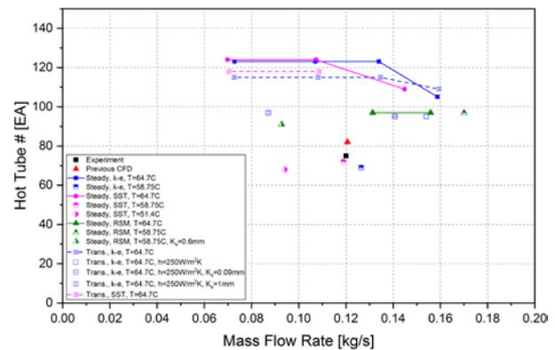
Fig. 5. Number of hot tubes according to hot leg mass flow rate
