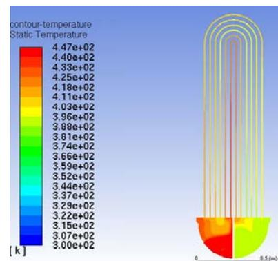
Fig. 9 Temperature distribution with no hot leg modeling
