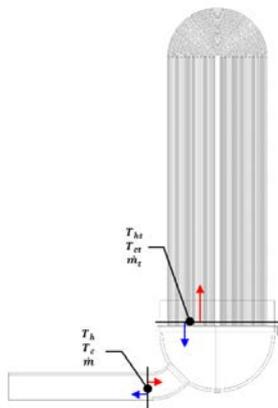
Fig. 4. Monitoring location for temperature and mass flow rate
