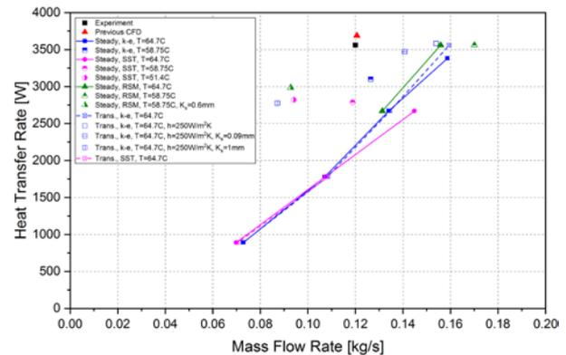
Fig. 6. Heat transfer rate at tube bundle according to hot leg mass flow rate
