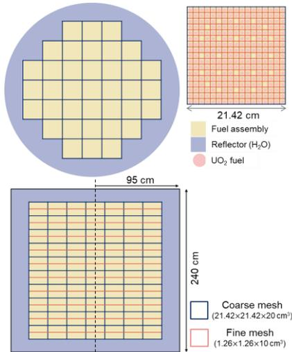
Fig. 3. Core configurations
