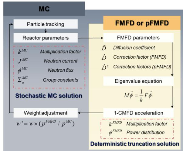
Fig. 1. Diagram of the FMFD and DTMC methods
