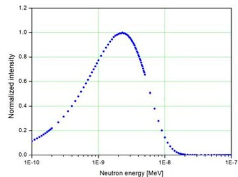
Fig. 1. Energy differential neutron flux of neutron beam
