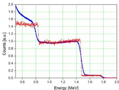
Fig. 4. Comparison of calculated and measured NDP spectra
