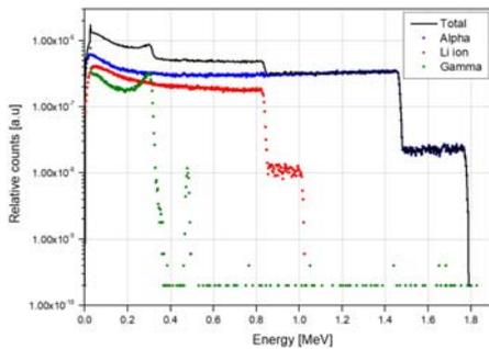
Fig. 3. Simulated neutron induced charged particle spectrum of SRM-93a
