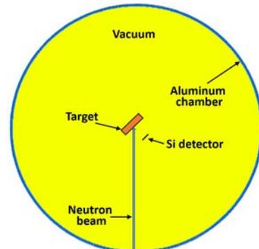
Fig. 2. Geometry of the MCNP model
