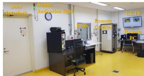
Fig. 2 MEVVA ion source safety system at control room
