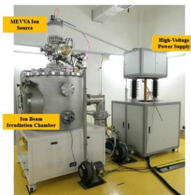
Fig. 1 The MEVVA ion beam facility at the KOMAC
