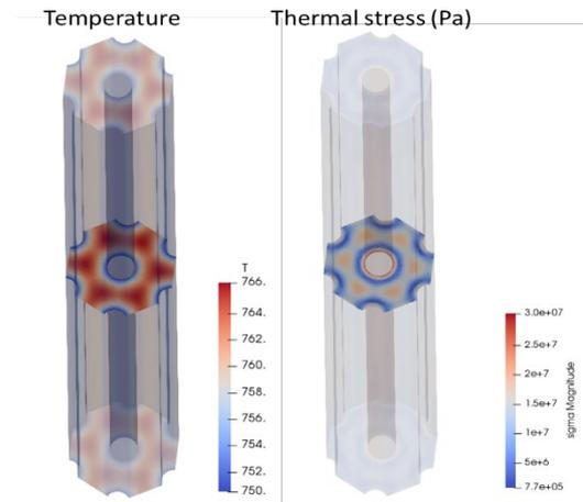
Fig. 8. Calculation result of the temperature and thermal stress for the unit cell problem.
