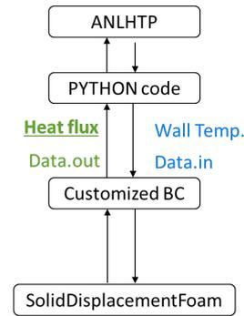
Fig. 3. Data transfer procedure of the ANLHTP-OpenFOAM coupled code.
