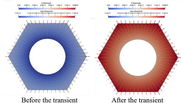
Fig. 5. Thermal stress and displacement vector in the coupled calculation.
