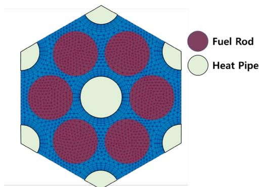
Fig. 7. Unit cell geometry and mesh of the OpenFOAM solver.
