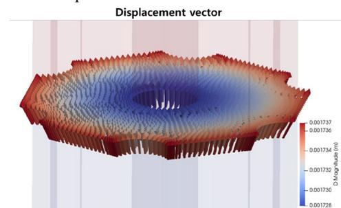
Fig. 9. Calculation result of the displacement vector for the unit cell problem.
