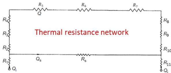
Fig. 2. Thermal resistance network of the ANLHTP code.
