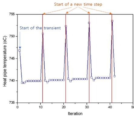
Fig. 6. Heat pipe wall temperature (during the transient) at each Picard iteration.
