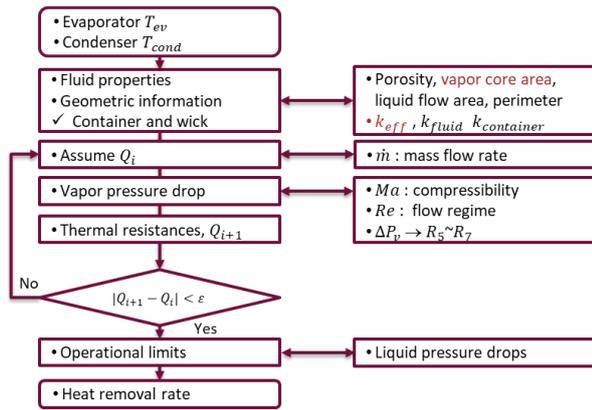
Fig. 1. Simplified calculation procedure of the ANLHTP code.
