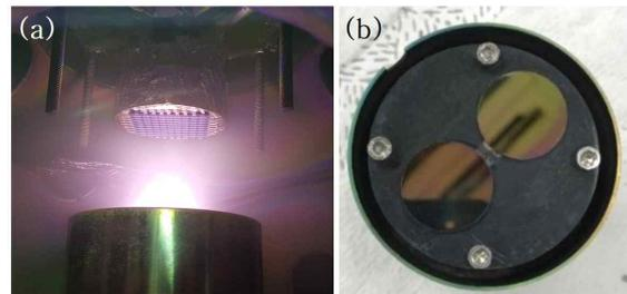
Fig. 6. The pictures of (a) RF sputtering and (b) B film on the Si substrate
