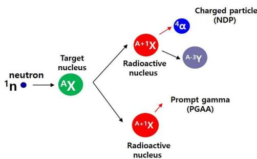
Fig. 1. A schematic diagram for NDP and PGAA
