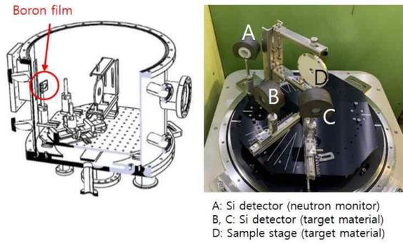
Fig. 4. The schematic diagram and picture of stage for KAERI-NDP system
