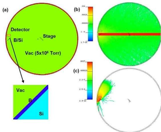
Fig. 5. (a) A model of target chamber on top view (b) neutron transmission ratio (91.1 %), (c) count rate of  $\alpha$  particles (4.15 cps)
