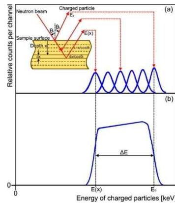
Fig. 2. A schematic diagram of energy distribution depending on depth  $x$  [1]
