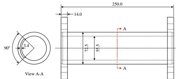
(a) Small-scale pipe specimen
