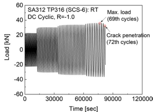
(b) Displacement-controlled multiple block load
