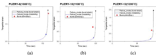
Fig. 4. Simulation results considering failure criteria; (a) PUZRY-8, (b) PUZRY-10, and (c) PUZRY-12.
