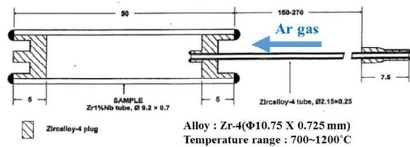
Fig. 2. Schematic drawing of the Zry-4 specimen for ballooning test at high temperature condition. [1]
