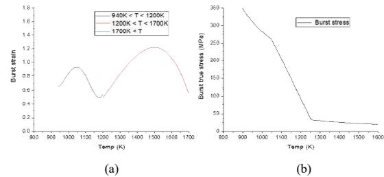
Fig. 1. Failure criteria at FRAPTRAN [4]: (a) Burst strain, (b) Burst stress
