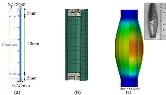
Fig. 3. Analysis model for PUZRY test; (a) axisymmetric model, (b) model rotated 270° in the axial direction, and (c) simulation results
