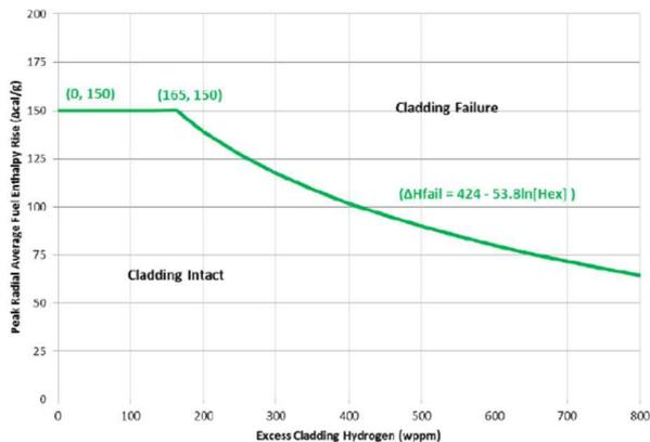
Fig. 1 PCMI Cladding Failure Threshold – SRA Cladding at High Temperature Reactor Coolant Conditions [2]
