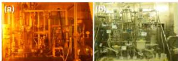
Fig. 3. Fission  $^{99}\text{Mo}$  Hot test production systems. (a) System for target dissolution installed in the irradiated material examination facility (IMEF) of KAERI. (b) System for  $^{99}\text{Mo}$  separation installed in the radioisotope production facility (RIPF) of KAERI.
