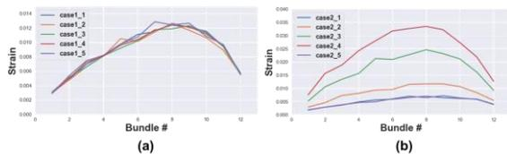
Fig. 3. Calculated tube expansion strains using randomly generated orientations from (a) the tube and (b) the generate texture information.
