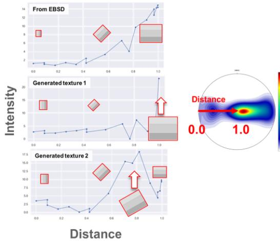
Fig. 2. Intensity profiles (left) along the line from the radial direction to the transverse direction as shown right pole figure. Top is of the tube and middle and bottom are of the generation process.
