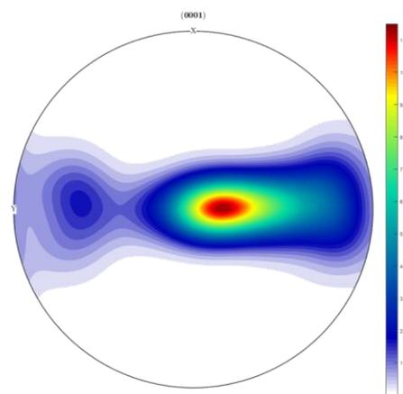
Fig. 1. Pole figure of (002) basal plane on the transverse plane where  $\hat{x}$ ,  $\hat{y}$  and  $\hat{z}$  axes indicates axial, radial and transverse, respectively.
