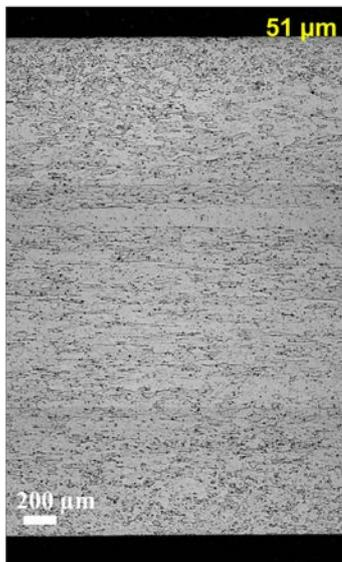
Fig. 1. Microstructure of Ti,Mo,C added 4th 136YTMC-2 alloy
