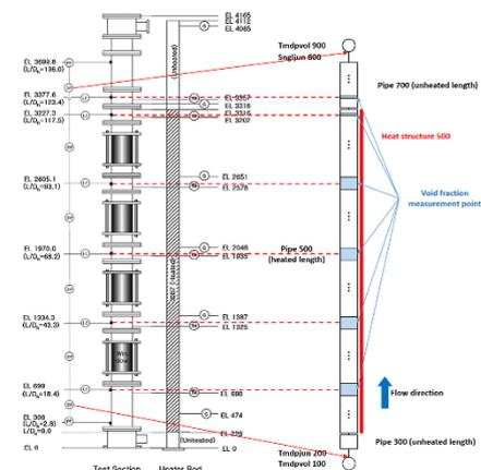
Fig. 2. SUBO input file nodalization
