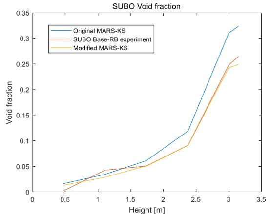
Fig. 5. Calculated void fraction of original MARS-KS, modified MARS-KS, and experimental data
