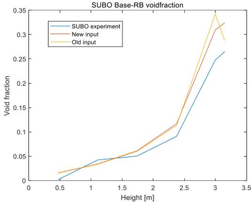
Fig. 3. Calculated Void fraction of Old input file and New input file
