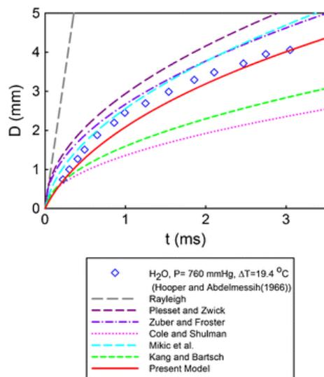
Fig. 1. Comparison of predicted rate of bubble growth by the presented model [2]
