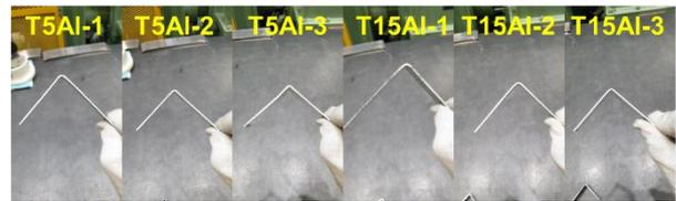
Fig. 6. Bending test results of U-5Al and U-15Al targets.
