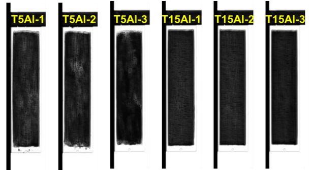
Fig. 5. Results of ultrasonic testing of U-5Al and U-15Al targets.
