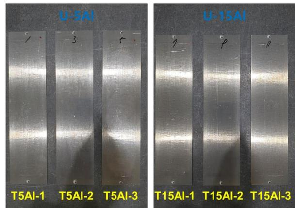
Fig. 2. Images of high-density U-5Al and U-15Al targets after the final machining.
