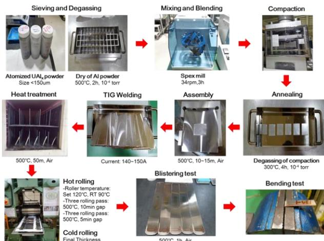
Fig. 1. Typical fabrication process of high-density targets [3].
