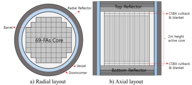
Fig. 6. The radial and axial ATOM core layouts
