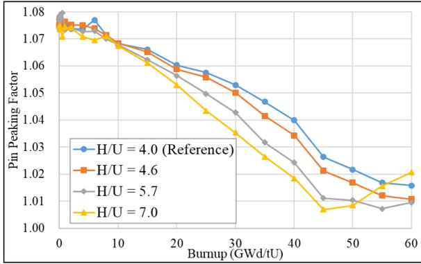
Fig. 5. Burnup-dependent PPF with respect to various H/U ratios
