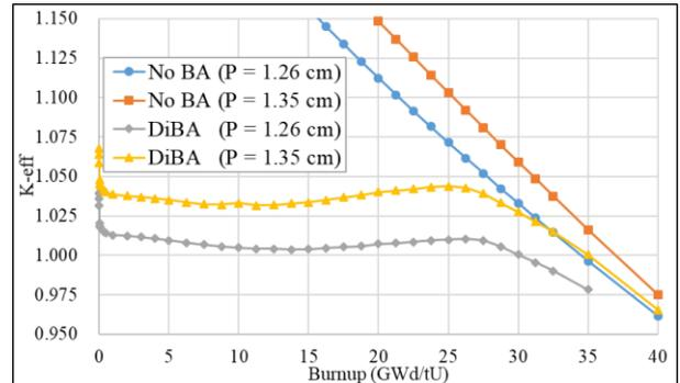
Fig. 9: Evolution of  $k_{eff}$  in various ATOM cores
