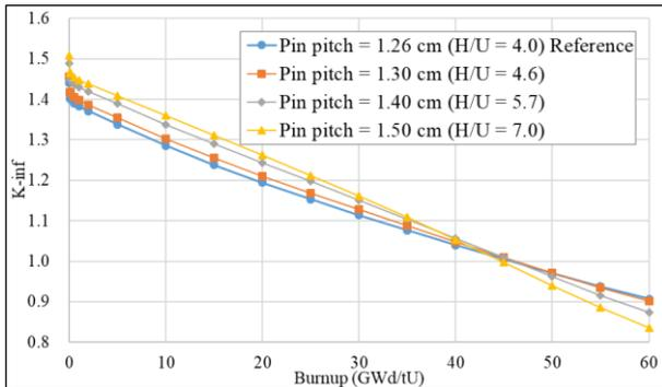
Fig. 3. The  $k_{inf}$  evolution for various initial H/U ratios
