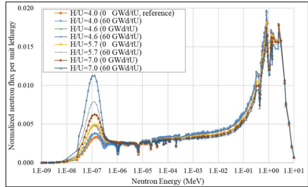
Fig. 4. Neutron spectrum with respect to various initial H/U ratio at 0 and 60 GWd/tU
