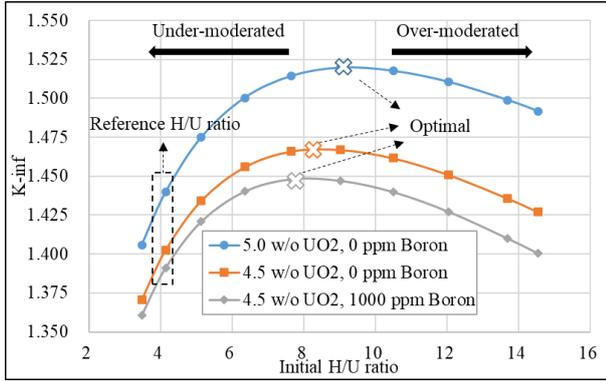
Fig. 2. The  $k_{inf}$  behavior with respect to H/U ratio.
