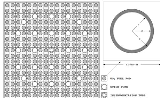
Fig. 1. 17x17 fuel assembly configuration
